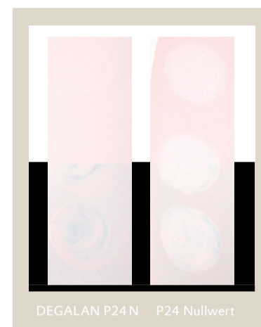
Figure 2: Rub-out test; Base formulations identical to figure 1; left: Base formulation 1 with continuously produced binder; right: Base formulation 2 with suspension polymer
